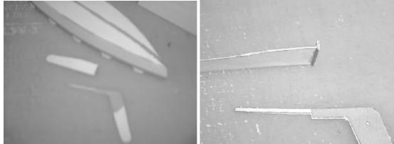
5. Assemble the rudder by folding the top piece over and gluing the lower piece in between. Assemble the daggar board by folding it over on itself and folding the top piece to form a stopper at the top.
